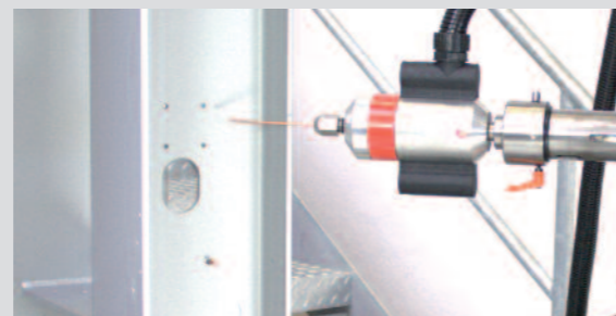
Erosion at any angle position or of large components
