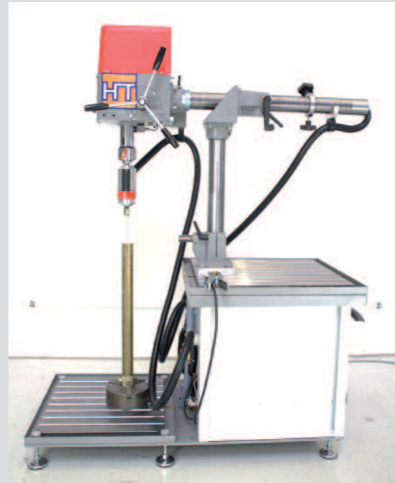
Erosion of large workpieces on the rear table of the static radial erosion unit
