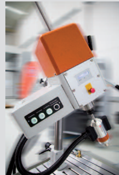
Erosion of slanting drill holes
