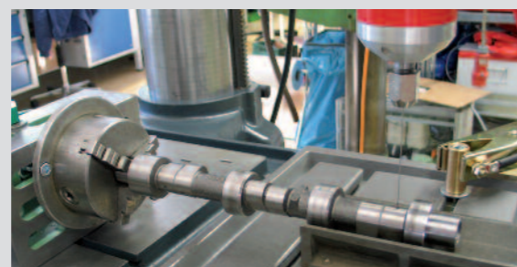
Erosion of a camshaft. Instead of the drill bit, the oscillating head of the erosion device is clamped in the machine
