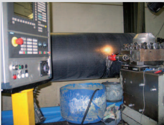
Horizontal erosion on a CNC lathe. The feed rate is regulated manually with the hand wheel
